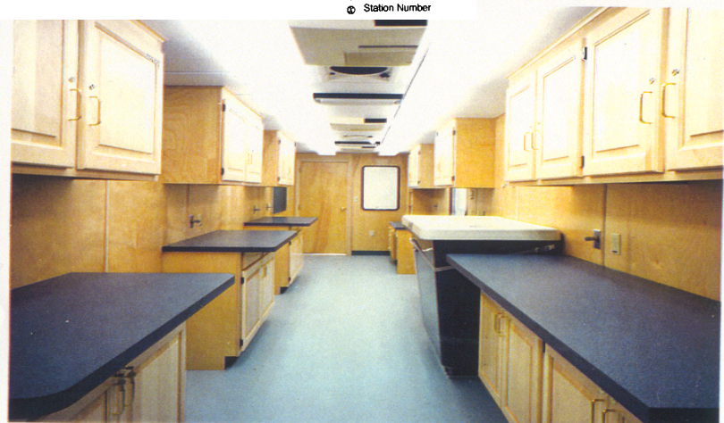
This 32 foot Voyager III Mobile Lab was delivered to Old Dominion University's College of Engineering and Technology, Norfolk, VA in July, 1998. The unit includes multiple analysis areas, overhead and under-counter storage, water weighing table for determination of flow rates, on-board air compressor for pneumatic air supply to each workstation, and a integrated computer system linking the student and teacher workstations.
