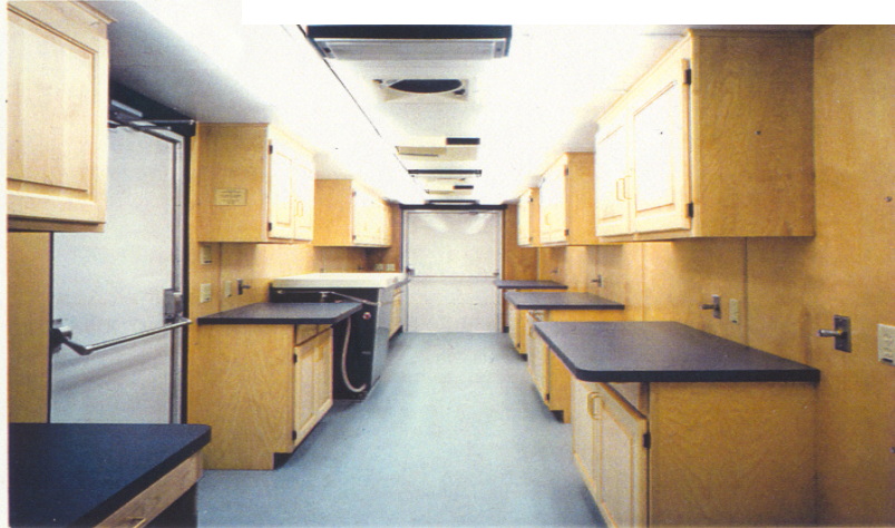
This 32 foot Voyager III Mobile Lab was delivered to Old Dominion University's College of Engineering and Technology, Norfolk, VA in July, 1998. The unit includes multiple analysis areas, overhead and under-counter storage, water weighing table for determination of flow rates, on-board air compressor for pneumatic air supply to each workstation, and a integrated computer system linking the student and teacher workstations.
